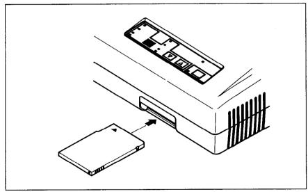
Figure 1-5. Slide the IC card into the front slot with the power switch off.
