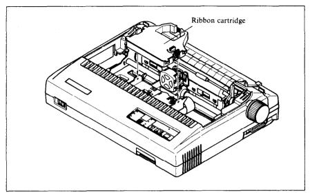
Figure 5-1. Replacing the ribbon cartridge
