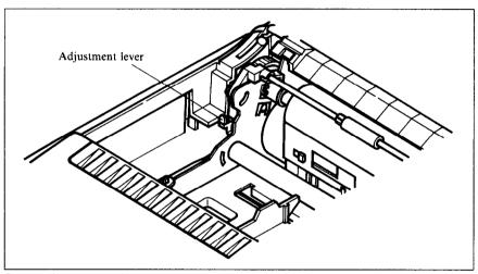
Figure 1-14. Adjusting for different thicknesses of paper
