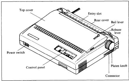
Figure 1-2. The printer's external parts
