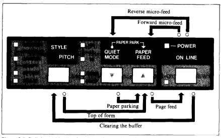
Figure 2-5. Switch combination functions of control panel
