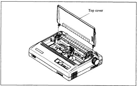
Figure 1-3. Removing the top cover
