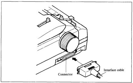
Figure 1-6. Connecting the interface cable
