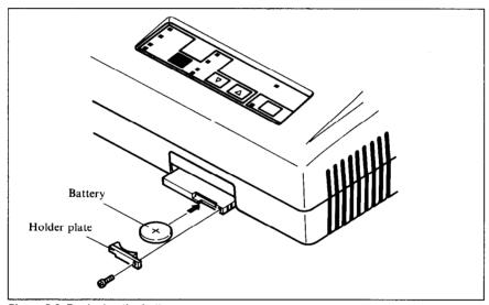
Figure 5-3. Replacing the battery
