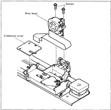
Figure 5-2. Replacing the print head
