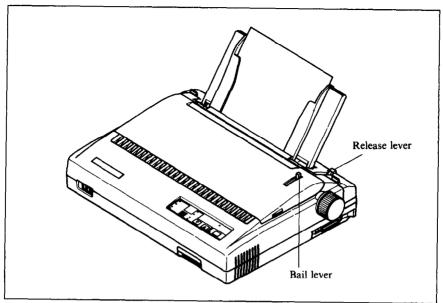
Figure 1-8. Loading a single sheet
