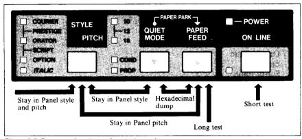
Figure 2-2. Power-up functions of control panel
