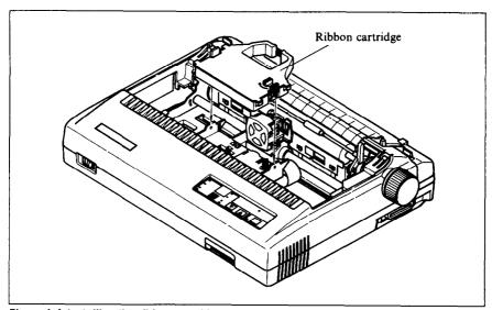
Figure 1-4. Installing the ribbon cartridge
