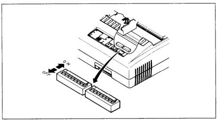
Figure 1-15. DIP switches
