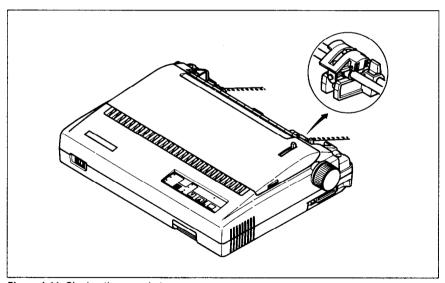
Figure 1-11. Closing the sprocket covers
