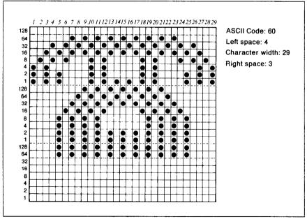
Figure C-1. Telephone symbol, Normal LQ pica
